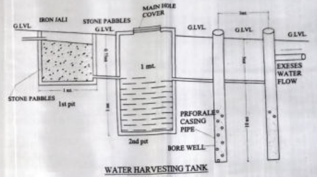
WATER HARVESTING TANK
